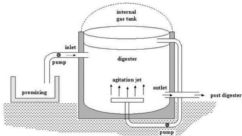
**Figure 1.** Biogas system including the anaerobic digester [11].
