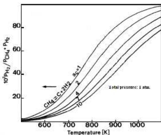
Fig. 2: Thermodynamic diagram showing isopotential curves for CH<sub>4</sub>-H<sub>2</sub> gas mixtures [55].
