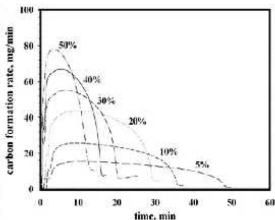
Fig. 9: Influence of methane concentration on carbon formation rate at T=800°C; mcat =25g; Q= 45Nl/h.
