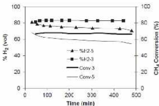
Fig. 6: Effect of catalyst amounts on production of hydrogen and CH<sub>4</sub> conversion.
