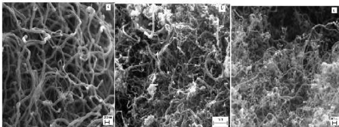
Fig. 12: SEM micrographs of as grown CNTs over the catalyst (a) catalyst 50%Ni-10%Cu-10%Zn/MCM-22 (b) catalyst 50%Ni-15%Cu-5%Zn/MCM-22, and (c) catalyst 50%Ni-15% Cu-15%Zn/MCM-22 after a CDM run at 750°C [163].
