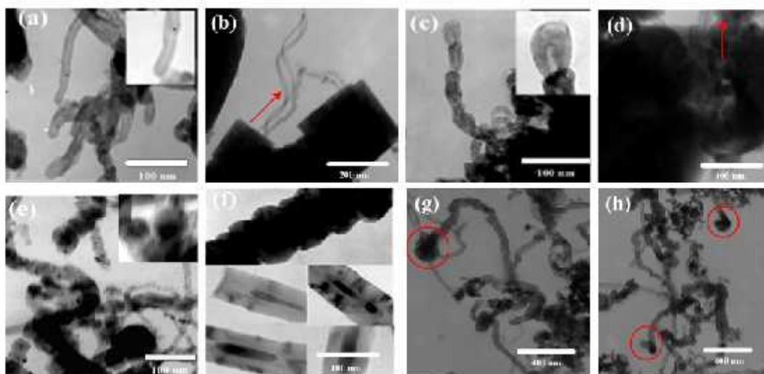
Fig. 11: Morphologies of carbon products over (a and b): HBETA zeolite; (c and d): HZSM-5 zeolite; (e–h):  $\text{Al}_2\text{O}_3$  (TEM graphs) [162].
