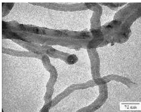
Fig. 13: TEM micrograph of the carbon deposit obtained on Ni<sub>30</sub>Cu<sub>50</sub> at 600 °C [164].
