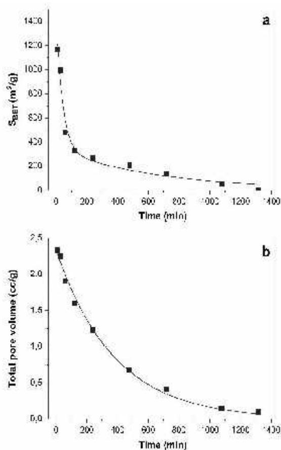
Fig. 10: Variation of the BET area (a) and total pore volume (b) against reaction time at  $T=950^\circ\text{C}$  and  $\text{GHSV}=360\text{ h}^{-1}$  [154].
