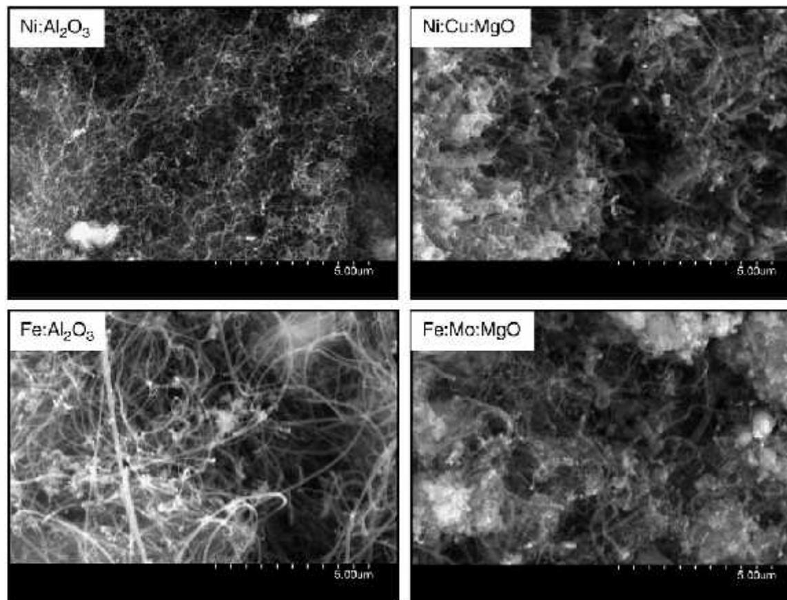
Fig. 14: SEM micrographs of the carbon nanostructures formed by CMD with each catalyst [30].
