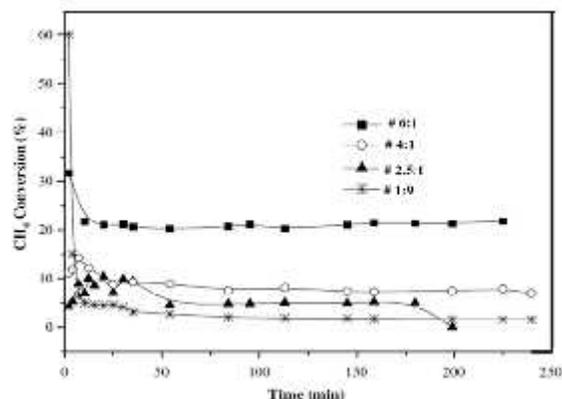
Fig. 7: Methane decomposition over 9-Co/Al<sub>2</sub>O<sub>3</sub> catalysts. Performance of the 9-Co/Al<sub>2</sub>O<sub>3</sub> catalyst in the CH<sub>4</sub> conversion with time-on-stream at 700 °C at different N<sub>2</sub>:CH<sub>4</sub> molar ratios.
