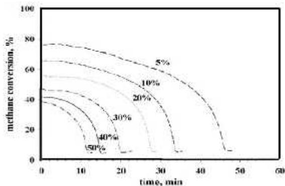
Fig. 8: Influence of methane concentration on methane conversion at T=800°C; mcat =25g; Q= 45Nl/h.
