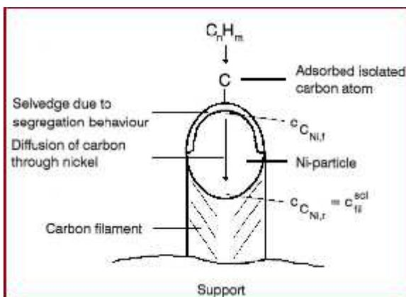
Fig. 3: Graphical representation of the mechanism of filamentous carbon formation [67].
