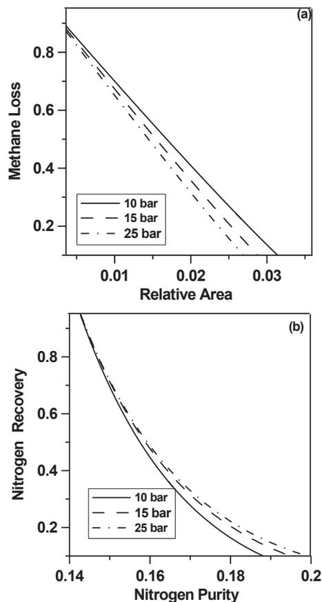
**Fig. 3.** Effect of feed pressure on the nanomembrane performance. Co-current configuration. Porosity is 0.36. Permeate pressure is 1 bar. Nitrogen in the feed is 14.14%.
