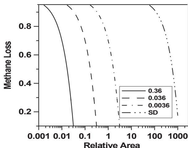
Fig. 4. Effect of porosity on the nanomembrane performance. Co-current configuration. Feed pressure is 10 bar. Permeate pressure is 2 bar. Nitrogen in the feed is 14.14%.
