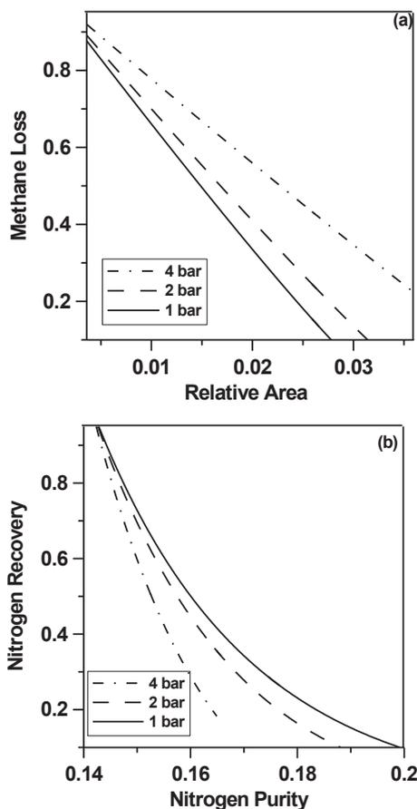
**Fig. 2.** Effect of permeate pressure on the nanomembrane performance. Co-current configuration. Porosity is 0.36. Feed pressure is 10 bar. Nitrogen in the feed is 14.14%.
