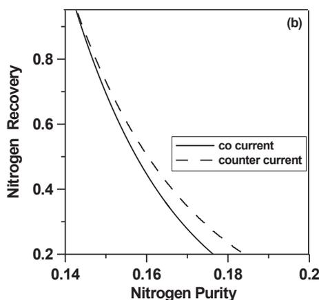
Fig. 5. Effect of flow configuration on the nanomembrane performance. Porosity is 0.36. Feed pressure is 10 bar. Permeate pressure is 2 bar. Nitrogen in the feed is 14.14%.
