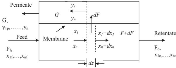
Fig. 1. Membrane flow diagram with counter-current flow.
