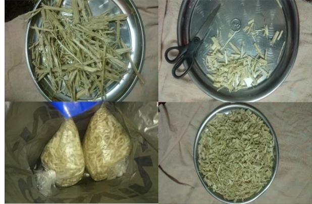
Figure 6. Cutting dried SCB
