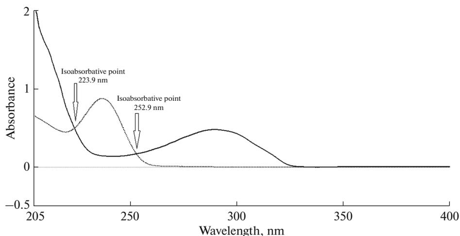
Fig. 1. Zero order absorption spectra of 10 µg/mL canagliflozin (—) and metformin (---) using methanol as blank.
