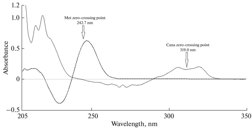
Fig. 3. Overlaid first derivative spectra of 10 µg/mL canagliflozin (—) and metformin (---) using methanol as blank.
