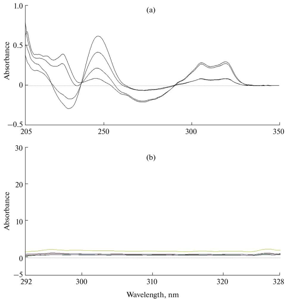
Fig. 4. First derivative absorption spectra of lab prepared mixtures with different canagliflozin (CANA) and metformin (MET) concentrations (a); CANA (5 µg/mL) as a divisor showing constants in the plateau region (292–382 nm) (b); different CANA concentrations (5–20 µg/mL) after constants multiplication by a divisor of CANA (5 µg/mL) (c); different MET concentrations (2–15 µg/mL) after subtraction of CANA first derivative absorption spectra (d).
