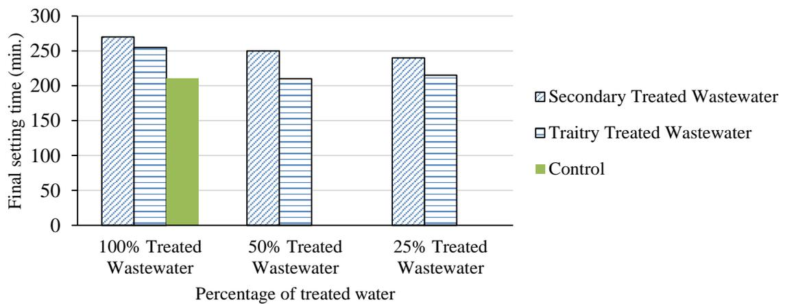
**Figure 2.** Final setting time for different wastewater percentages.
