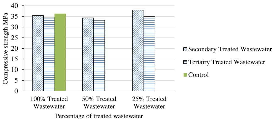
**Figure 4.** Compressive strength of concrete cube specimens at age of 28 days.
