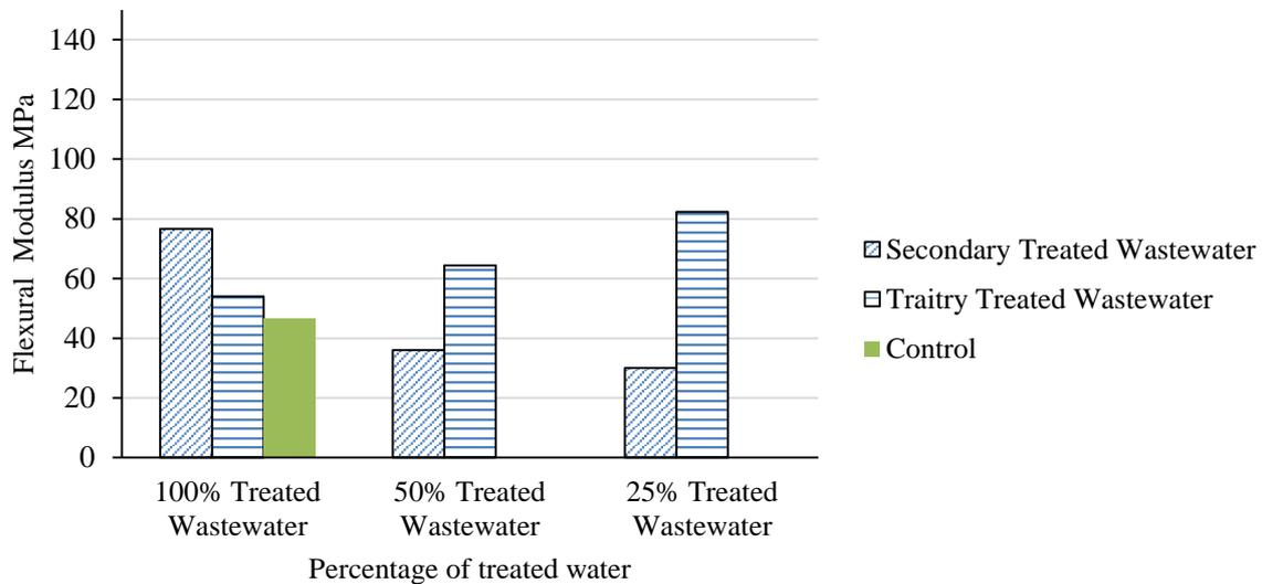
**Figure 5.** Flexural modulus at age of 7 days.
