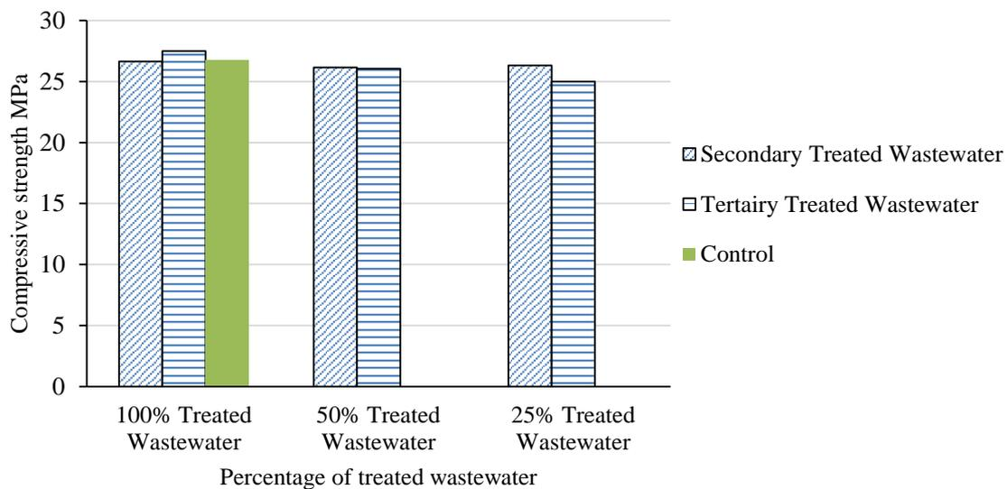
**Figure 3.** Compressive strength of concrete cube specimens at age of 7 days.
