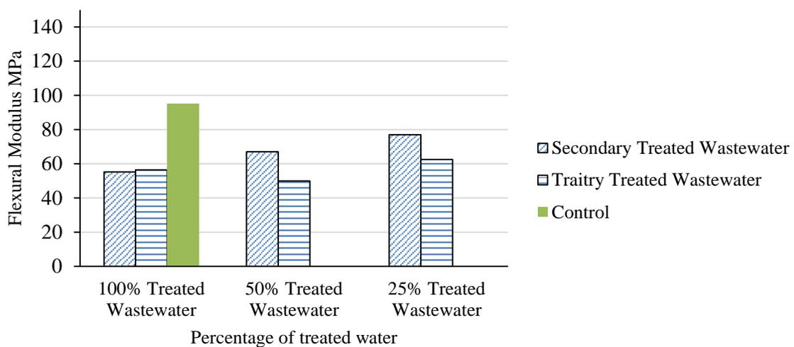
**Figure 6.** Flexural modulus at age of 28 days.
