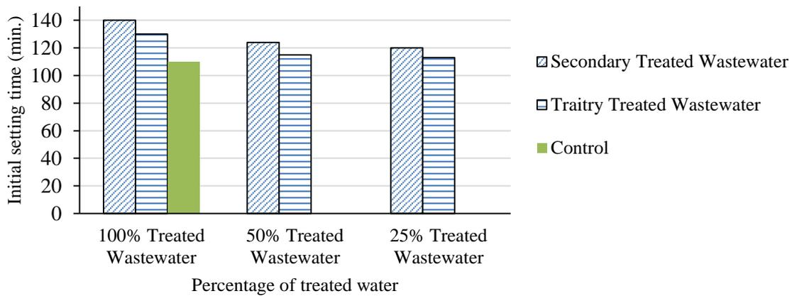
**Figure 1.** Initial setting time for different wastewater percentages.
