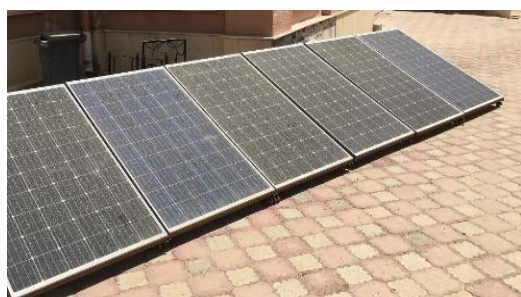
Figure 3: Tested solar panels held on 30^\circ tilted holders facing South direction.
