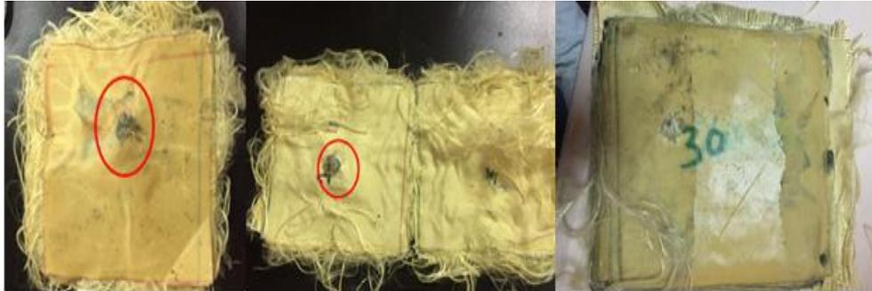
**Fig. 1:** Penetration Tests Showing Holes Formed for Samples 1, 2, and 3 Respectively.
