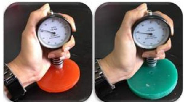
**Fig. 5:** Hardness Shore D Test.
