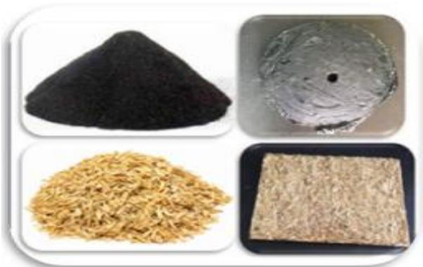
**Fig. 1:** Automobile Tire Power and Rice Husk Mixed with Epoxy Preparation.
