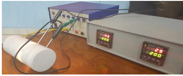
Fig. 6: Thermal Insulation Measuring Device.
