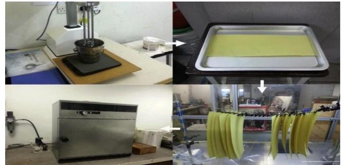
**Figure 1. The preparation process of a ballistic fabric sample impregnated in a shear thickening fluid (STF) (Gurgen, Kushan, & Li, 2017)**
