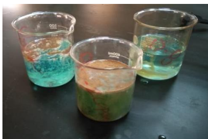
Figure 1: Effect of adding Hydrazine hydrate on copper and chitosan solution
