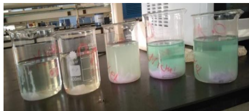
Figure 2: Effect of adding Hydrazine hydrate on Nickel and chitosan solution
