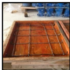
Figure 1 (left) Wooden mold of slab and steel arrangement
