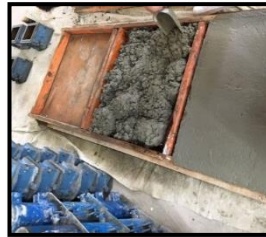
Figure 1 (left) Wooden mold of slab and steel arrangement
