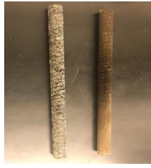
Figure 5 BFRP before (left) and after (right) heating.
