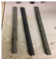
Figure 6 Steel, CFRP, BFRP (left to right) after heating
