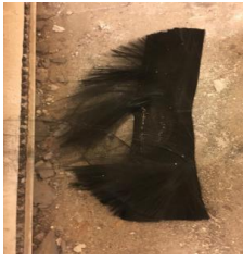
Figure 4. CFRP bars after 2 hours at 600°C
