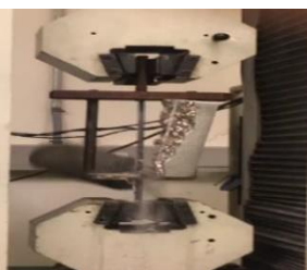
Figure 7 CFRP reinforced cylinder
