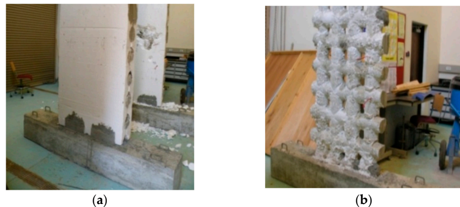
Figure 8. Constituents of Wall W_2 : (a) With EPS cover; (b) Without EPS cover.
