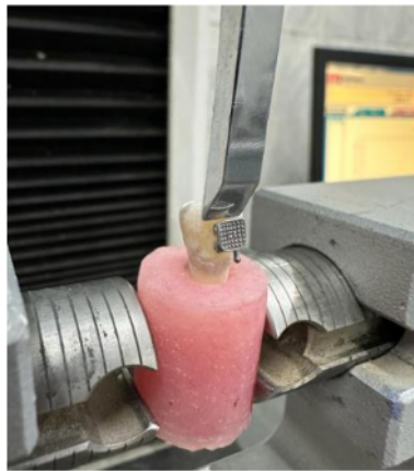
Figure (1): Shear bond strength test.
