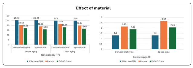
The conventional sintering cycle produced significantly higher TP than speed cycle for both Katana UTML Zirconia (P < 0.001) and IPS e.max ZirCAD Prime (P < 0.001) when measured before and after aging. Conventional sintering cycle induced a significantly lower change in color for Katana UTML Zirconia (P = 0.004) when compared with the speed sintering cycle while the change in color of IPS
