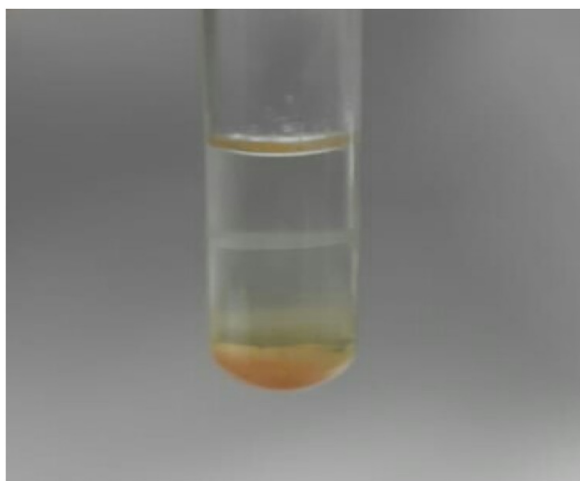
Fig. 3. Show the effect of freezing lipid precipitation approach on precipitation of 1.0 mL human plasma by 1.0 mL Acetonitrile, vortex 30 sec. and freezing 10 min at -80^{\circ}\text{C} followed by Centrifugation 5.0 min at 4200 \times g (Layers from bottom to top precipitate of plasma protein, precipitate of plasma lipid and bile pigments, slightly turbid layer with plasma lipid and very clear layer used for analytes determination).
